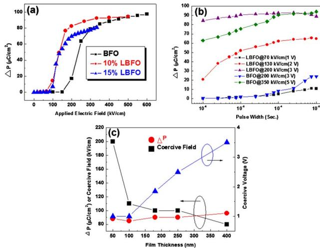
FIG. 4. (Color online) Switched polarization ( $\Delta P$ ) as a function of (a) applied electric field and (b) pulse width. (c) Thickness dependence of the ferroelectric properties ( $\Delta P$ , coercive field and voltage).
