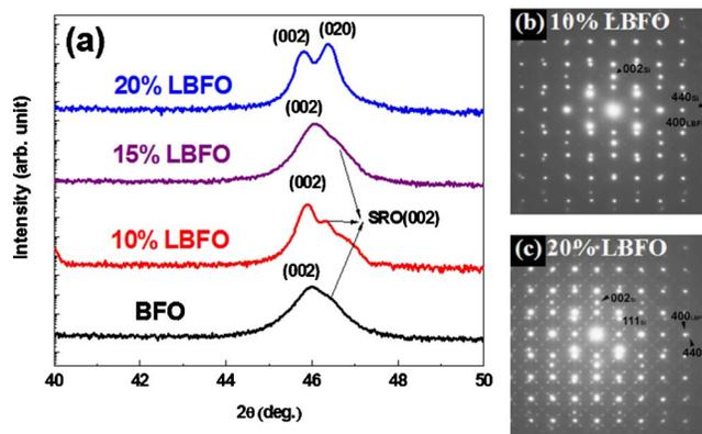
FIG. 1. (Color online) (a) Typical x-ray  $\theta$ - $2\theta$  scans of the BFO and LBFO films with different La concentrations on SRO/STO/Si substrates. Electron diffraction patterns of (b) 10% and (c) 20% LBFO films.
