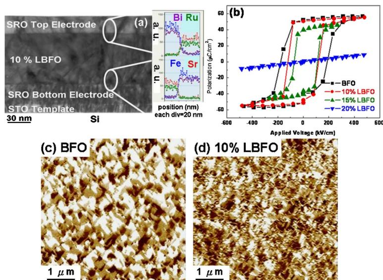
FIG. 3. (Color online) (a) Cross-sectional TEM image and energy dispersive spectroscopy of SRO/LBFO/SRO/STO/Si films. (b)  $P$ - $E$  hysteresis loops, of BFO and LBFO films with different La concentrations. As grown ferroelectric domain structures of (c) BFO and (d) 10% LBFO films.
