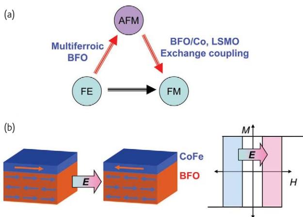
Fig. 5 An approach for the electrical control of ferromagnetism. (a) Schematic of our method for electrical control of magnetism. The connection between ferroelectricity (FE), antiferromagnetism (AFM), and ferromagnetism (FM) is shown. (b) Schematic showing the use of BFO films to control the ferromagnetism in CoFe via an exchange-coupling interaction.
