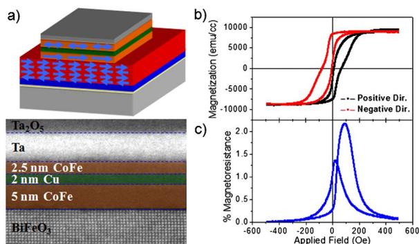
FIG. 3. (Color online) Spin valve structures based on CoFe/Cu/CoFe/BFO heterostructures. (a) Schematic illustration and scanning transmission electron microscopy image (b) Magnetic hysteresis loops of spin valve structures. (c) Current-in-plane magnetoresistance measurements.
