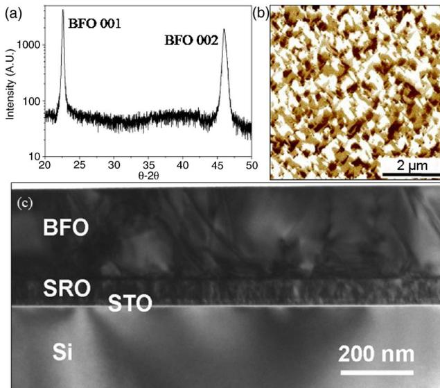
FIG. 1. (Color online) Structural analysis of typical  $\text{BiFeO}_3$  films on Si (001) substrates. (a) X-ray diffraction. (b) In-plane piezoforce microscopy image shows the presence of all four in-plane polarization variants in these BFO films. (c) Transmission electron microscopy image.
