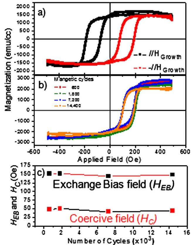
FIG. 2. (Color online) Typical magnetic properties for bilayer CoFe/BFO heterostructures. (a) Magnetization hysteresis loops reveal large negative exchange bias. (b) Repeated magnetic cycling results in very little change in the magnetic properties. (c) Exchange bias field and coercive field as a function of magnetic cycle—no training effect is observed.
