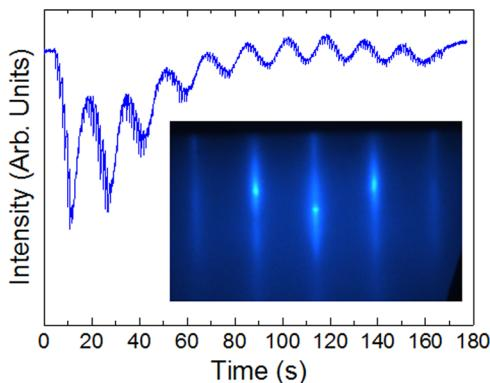
FIG. 1. RHEED-assisted growth of a 10 unit cell thick LaAlO<sub>3</sub> film on a SrTiO<sub>3</sub>(001) substrate. Clear oscillations in the intensity of the specular RHEED spot reveal layer-by-layer growth (where each individual laser pulse is evident within the oscillations). The inset shows the RHEED pattern immediately following growth and is indicative of a very smooth film surface.
