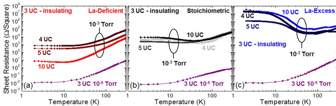
FIG. 3. Sheet resistance as a function of temperature and film thickness (3, 4, 5, and 10 uc) for  $\text{LaAlO}_3/\text{SrTiO}_3(001)$  heterostructures, where the  $\text{LaAlO}_3$  was controlled to possess (a) 4%–5% La-deficiency, (b) nearly stoichiometric, and (c) 4%–5% La-excess film stoichiometry at a growth pressure of  $10^{-3}$  Torr of oxygen. For comparison, the sheet resistance of a film of like stoichiometry, but grown at  $10^{-6}$  Torr (purple data), is provided in each panel.
