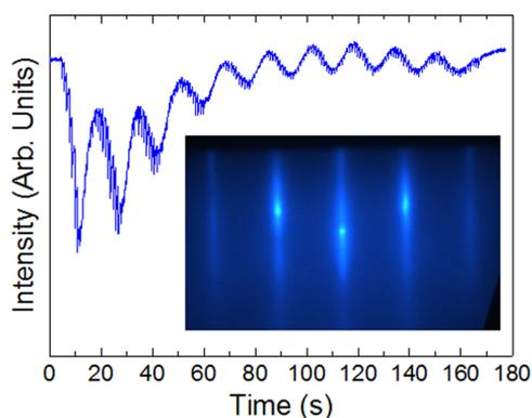
FIG. 1. RHEED-assisted growth of a 10 unit cell thick LaAlO<sub>3</sub> films on a SrTiO<sub>3</sub>(001) substrate. Clear oscillations in the intensity of the specular RHEED spot reveal layer-by-layer growth (where each individual laser pulse is evident within the oscillations). The inset shows the RHEED pattern immediately following growth and is indicative of a very smooth film surface.
